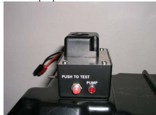
Front view of control unit with push to test button and pump active LED visible
